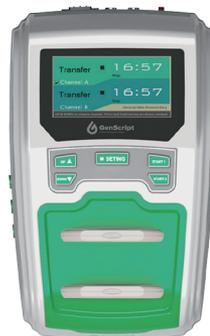
**Step 5.** For Channel A, push "Start A" button, and it will start flashing. The timer on the screen will begin the countdown. Machine will beep when the countdown reaches 0, push "Start A" again to finish the process. For Channel B, push "Start B" and follow similar procedure as above.
