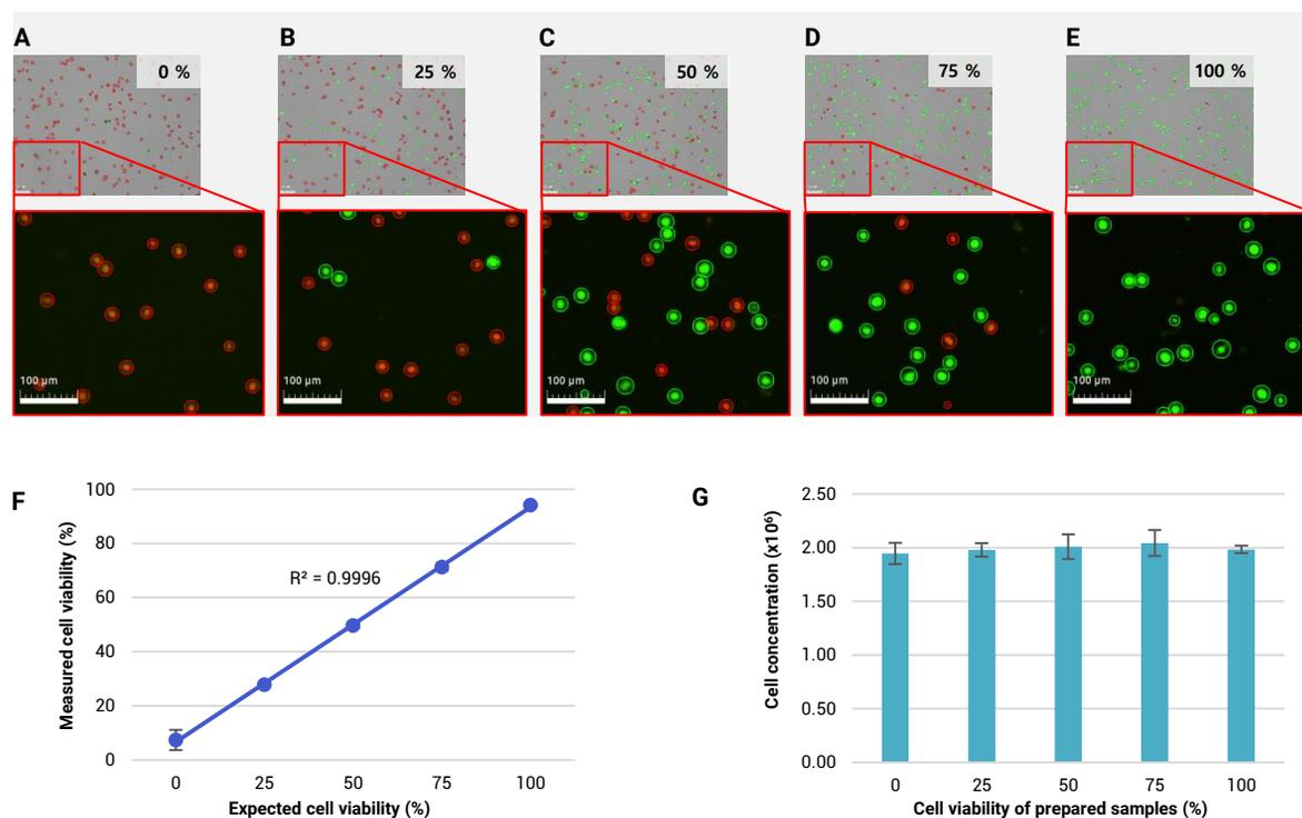
**Figure 2.** The linearity of the LUNA-FX7™ in dual fluorescent counting. Cells were counted in Fluorescence Cell Counting mode using AO/PI dye. (A-E) Tagged images of 0, 25, 50, 75 and 100% viability. (F) Measured viability of K562 plotted against expected viability. (G) Measured total cell concentrations at five different viability samples are steady and not significant.
