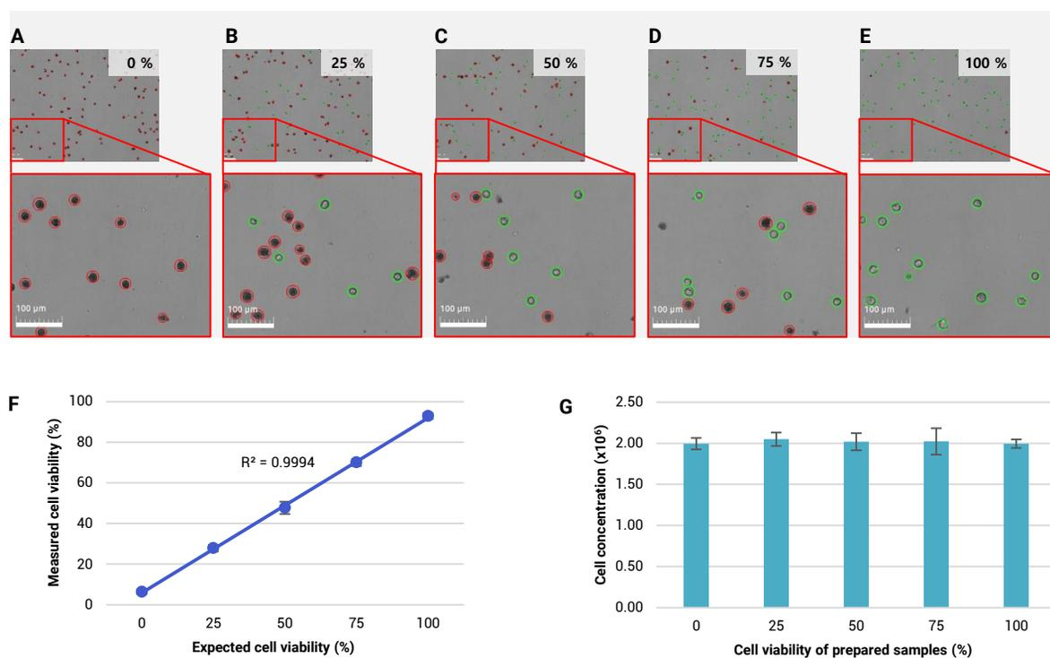
**Figure 1.** The linearity of the LUNA-FX7™ in brightfield counting. Cells were counted in Brightfield Cell Counting & Viability mode using Trypan blue staining. (A-E) Tagged images of 0, 25, 50, 75 and 100% viability. (F) Measured viability of K562 plotted against the expected viability. (G) Constancy of the total cell concentrations at five different viability samples.
