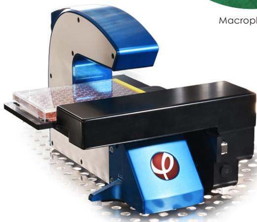
**HoloMonitor® is a live cell imaging system designed to visualize and quantify adherent cells over time. It is gentle to all cell types and can be used to monitor cell lines as well as delicate cell types, such as induced pluripotent stem cells or primary human cell cultures. As cell imaging with HoloMonitor is label-free and harmless to your cells, the cells can be used for further studies after imaging.**
