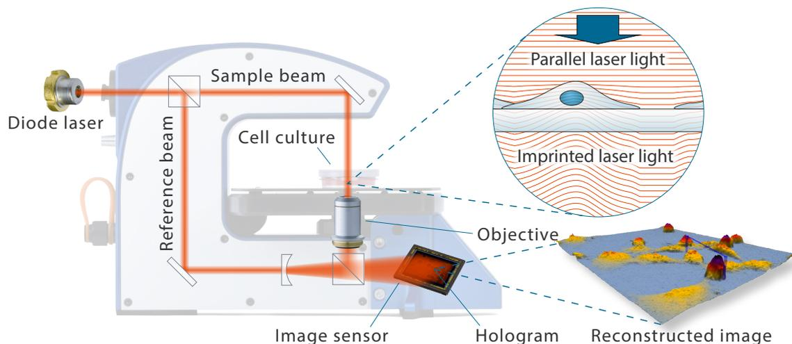
Holographic microscopy creates quantitative phase images by letting a sample beam and a reference beam interfere to generate an interference pattern – the hologram.
